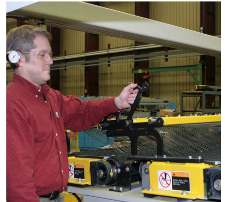
Retaining clamp quickly pivots away.
