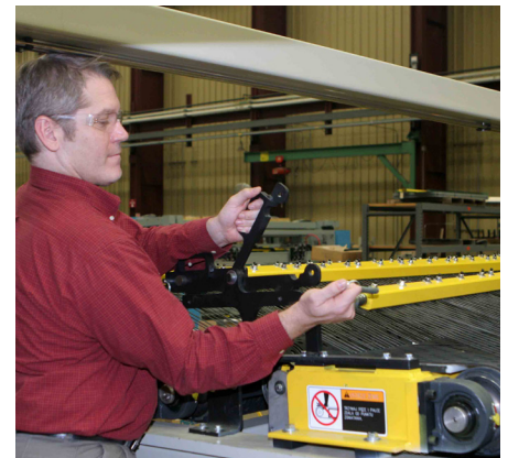
Brush assembly is easily removed.
