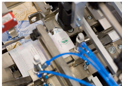
Page scanner to verify opening
