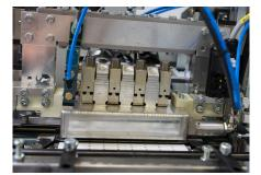
PUR gluing nozzle
