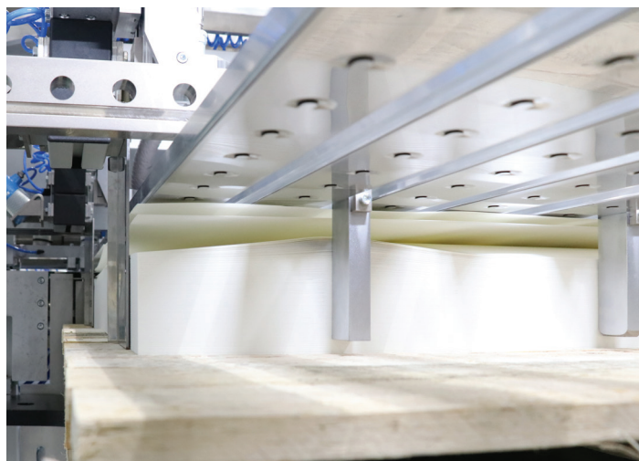
Material almost gaplessly guided and under permanent tension.
