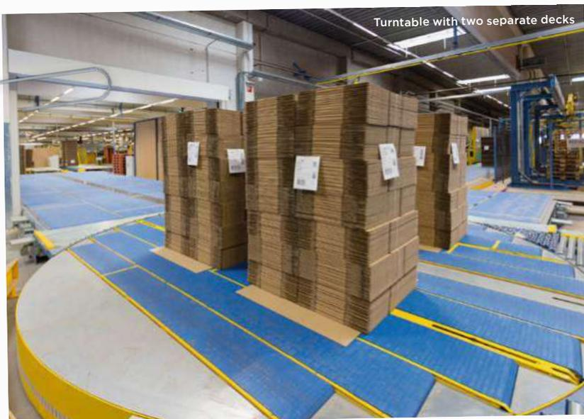
Turntable with two separate decks
