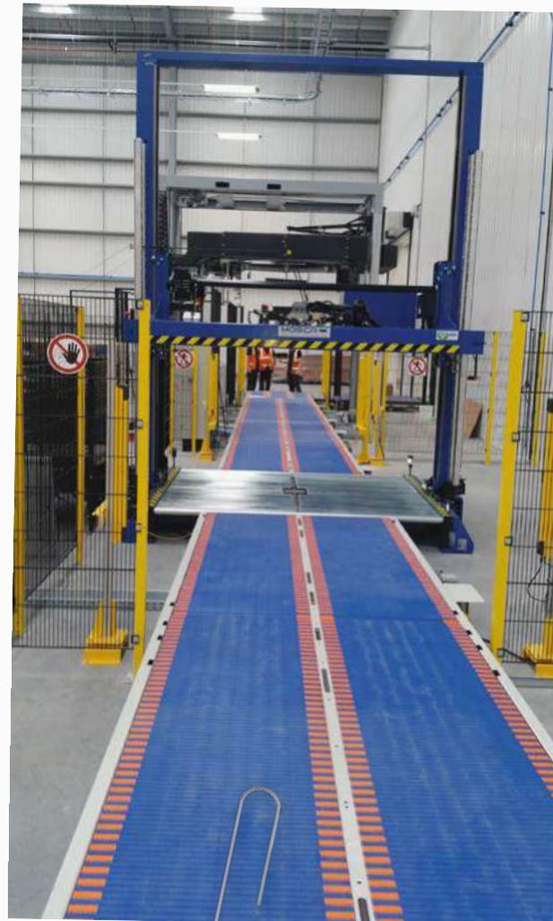
is fully automatic and requires less space than a traditional pre-feeder. In addition installations benefit from IMS conveyor equipment, control and guarding systems which ensures UK standards and support are provided.
