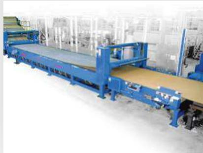
down force needed to bond the papers. The pulling was done by a Vacuum Traction Section (VTS). This combination of technologies allowed the board to cure faster, have better strength characteristics and have a low cost of ownership.
