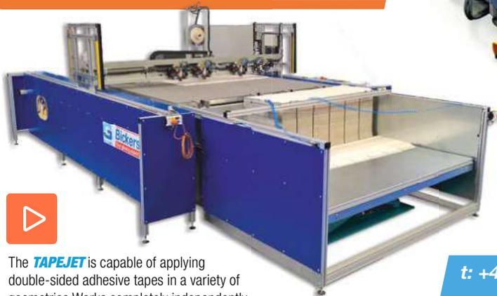
The **TAPEJET** is capable of applying double-sided adhesive tapes in a variety of geometries. Works completely independently using pick-and-place.
