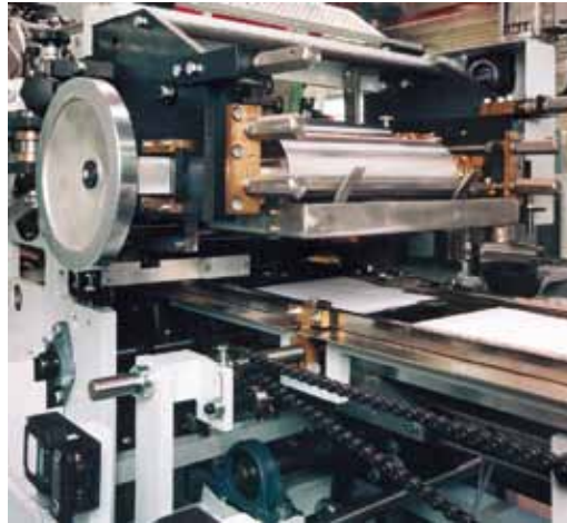
Figure 2 Sewn book block, to be bonded onto the passport cover, about to enter the bonding module of a Kugler-Womako passport line (source: Kugler-Womako).
