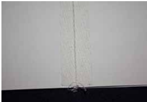
Figure 3 Book block of a passport with reinforcement tape, bonded across the spine of the endpaper.
