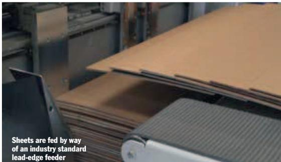
Sheets are fed by way of an industry standard lead-edge feeder
